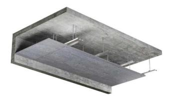
Valchromat panels are suitable to be used as a covering element for a false ceiling. The support structure will be made of galvanized steel or wood, with equidistant supports, whereby the distance should not exceed 600mm (24").
