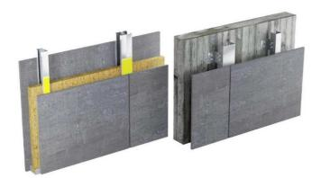
Valchromat panels can be used to make partition walls or interior wall cladding. When applied to interior partition walls they can be varnished or installed without finishing. It is the installer's responsibility to check the safety conditions of the support structure, namely the distance between supports and the width of the supports for proper panel installation.
