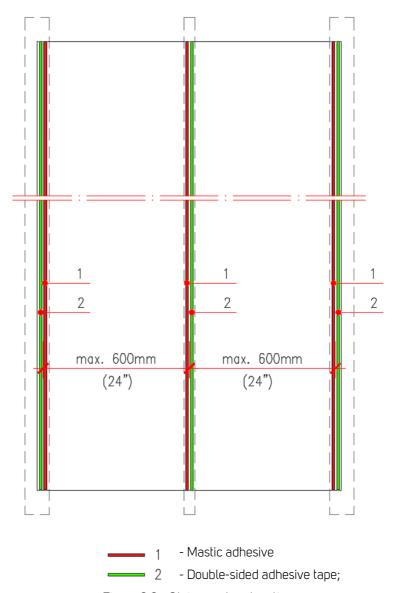
Figure 2.2 - Gluing system location
