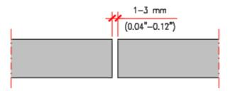
Figure 2.24 - Joints between panels
