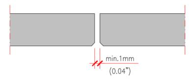
Figure 4.9 – Bevelled edge
