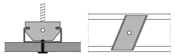
Figure 4.6 - Panel attachment detail to the support section
