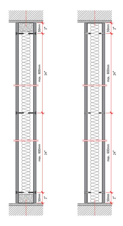
Figure 2.18 - Vertical section of the wall Structure, wood, and galvanized steel
