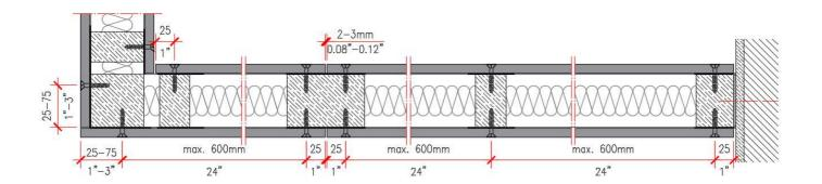
Figure 2.16 - Horizontal section of the wall, wooden structure
