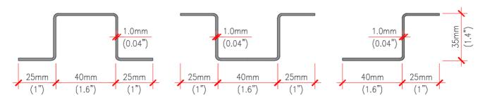
Figure 2.20 - Section type of structure in galvanized steel DX51D (Z+) (Dx51D Z+ galvanized steel)
