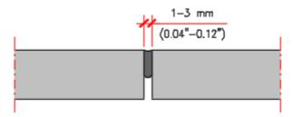
Figure 3.14 - Joints between panels with mastic
