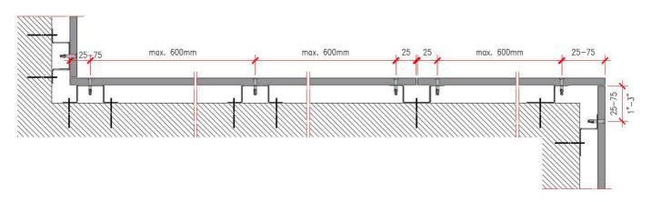
Figure 2.22 - Horizontal section, galvanized steel structure
