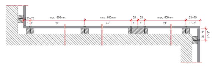
Figure 2.21 - Horizontal section, wooden structure
