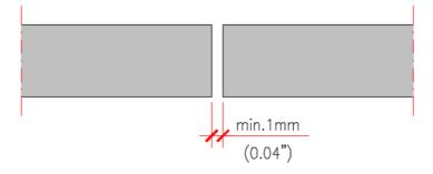
Figure 4.8 - Joint between panels
